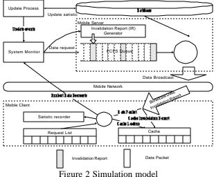
Figure 2 Simulation model
